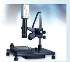
The instrument is designed and developed for quick checking of die bore sizes with the help of an optical image and customised measuring software.
