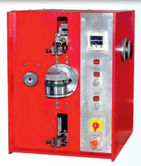
This machine is designed and developed for sizing and polishing of polycrystalline, natural and Mono diamond dies of size range from 0.100mm to 10.00mm. The machine is specially designed for the RBD sizes of range 2.500 mm to 10.00 mm.
