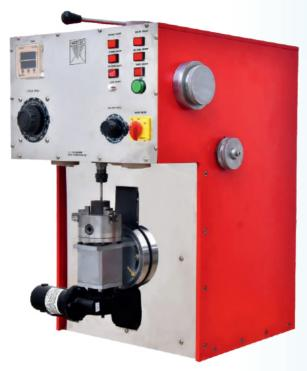
The machine is designed and developed for working of reduction and bearing portions of the Tungsten carbide dies. Also the machine can be used for working special tools, extruder dies, round bores of hard metals etc.
